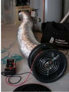
*Duct Leakage to Outside*
